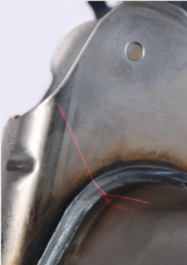
Weld seam inspection on a steel component
