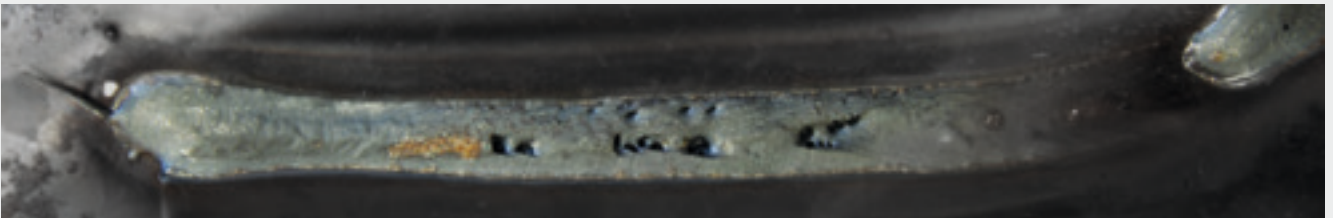
Hollow weld with pores
